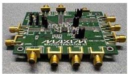
Objective: To verify the performance of this dual-band triple-mode CDMA front-end IC using a common, digital, 85MHz IF SAW filter and an 85MHz AMPS FM IF SAW filter.
